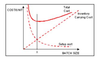
In the above diagram, it is shown that the x-axis is batch size and the cost of a unit is on the y-axis. It is shown that with the increase in batch size holding costs also tend to increase whereas setup costs tend to decrease. The point where both the cost line intersects each other signifies the lowest cost combination. The objective is to determine the batch size that developed on both sets of formulas.
